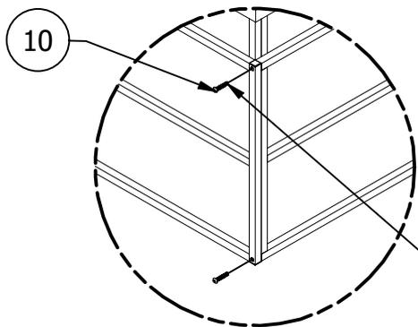
Secure main shell to side shell with (2) 3/8-16x2 bolts using a 7/32 Hex Drive.
